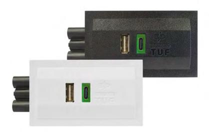
The new QF15 TUF HP module incorporates our latest evolution in high power USB charging. With its 65W maximum output QF15 TUF HP can provide up to 65W through the USB Type-C port, for high speed USB PD laptop, phone and tablet charging, whilst still allowing fast charging through the USB Type-A port for older devices.
